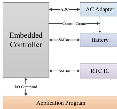
Fig. 1. System architecture of the EC and application program.
