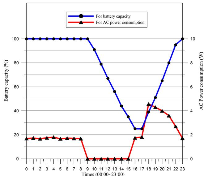
Fig. 4. Power consumption measurements of the peak-shift control method.
