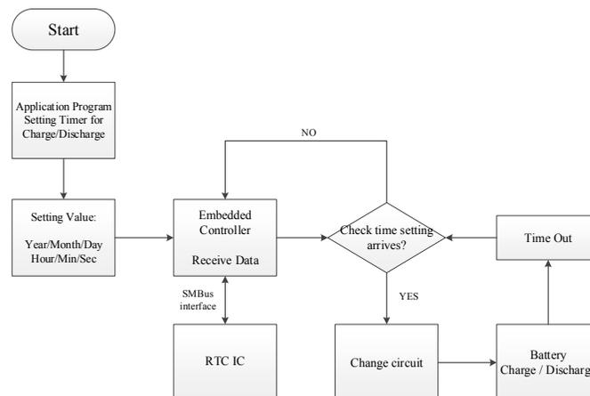
Fig. 2. Flowchart of the peak-shift control method.
