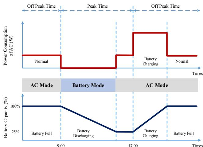
Fig. 3. Power consumption of the peak-shift control method.
