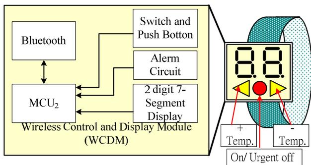
Fig. 4. Block diagram of WCDM
