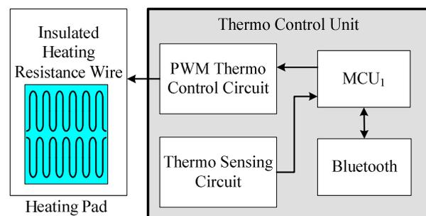
Fig. 3. Hardware architecture of thermo control unit and heating pad.
