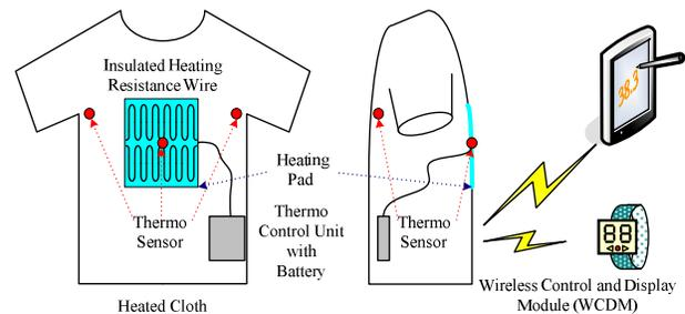
Fig. 2. Concept of the heated clothing overheating.
