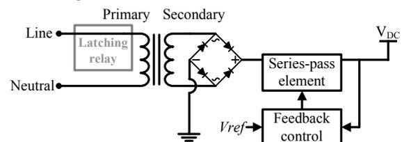
Fig. 1. Block diagram of the linear regulator.
