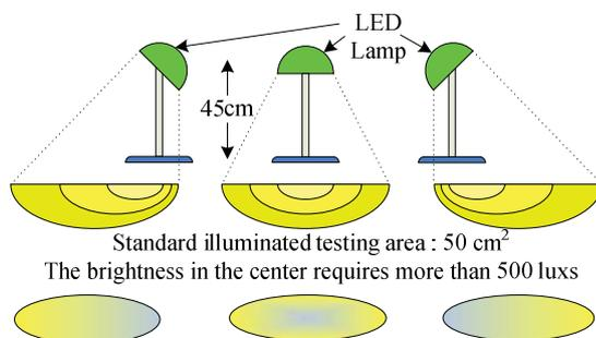
Fig. 1. The relation between the lamp shade rotation angle and the illumination areas
