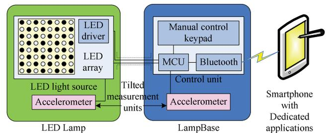
Fig. 2. The halftone digital LED desk lamp system diagram
