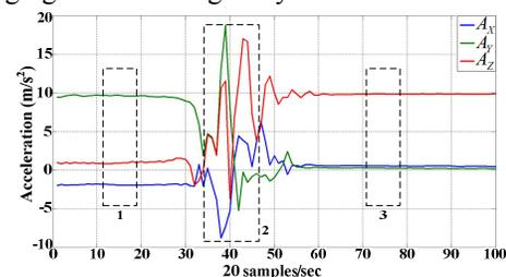
Fig. 2. Falling acceleration waveform.
