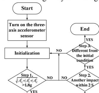
Fig. 3. The fall detection flowchart.
