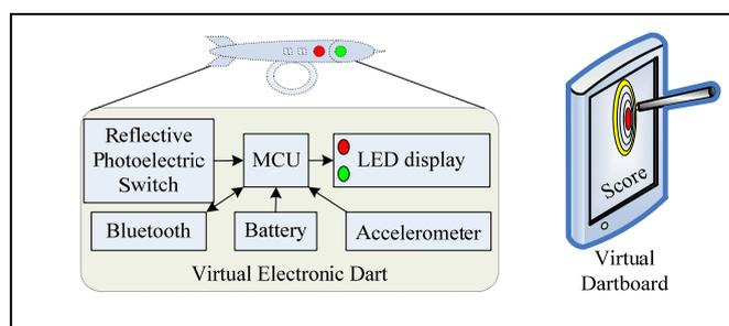
Fig. 1. The virtual electronic dart hardware architecture.
