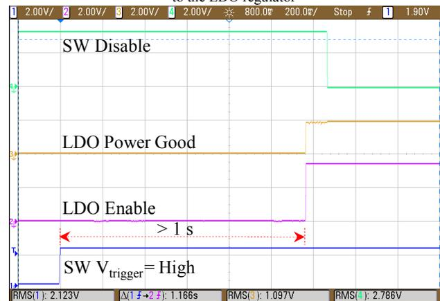
Fig. 11. The MCU controls the switching regulator swap to the LDO regulator waveform
