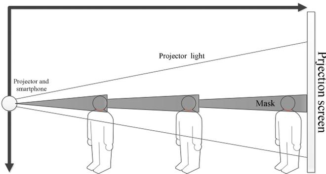
Fig. 8. The mask can automatically change size to protect the speaker's eye.
