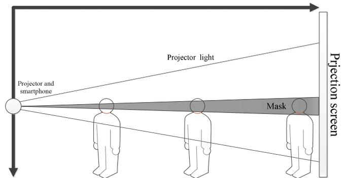
Fig. 7. The identical mask radius at the same distance between the projector and the screen.
