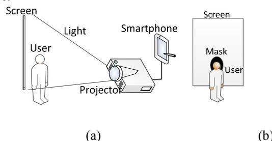
Fig. 1. Hardware architecture.
