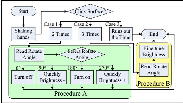
Fig. 3. The hand gesture detection flowchart.
