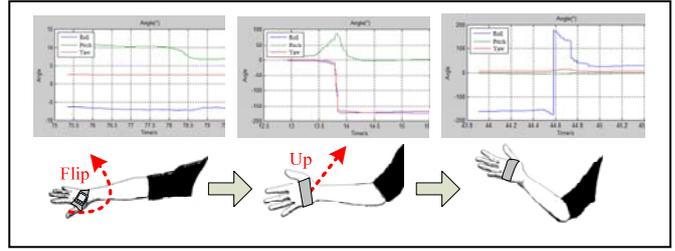
Fig. 4. The relationship between the hand and the sensor signals
