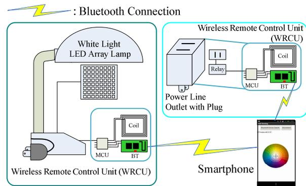
Fig. 1. The hardware architecture.
