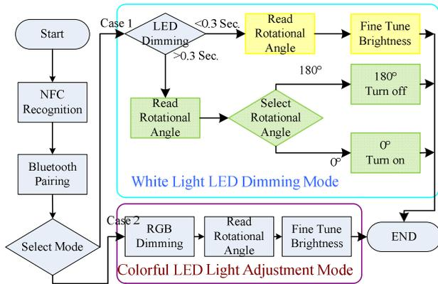
Fig. 2. The smartphone application software flowchart.
