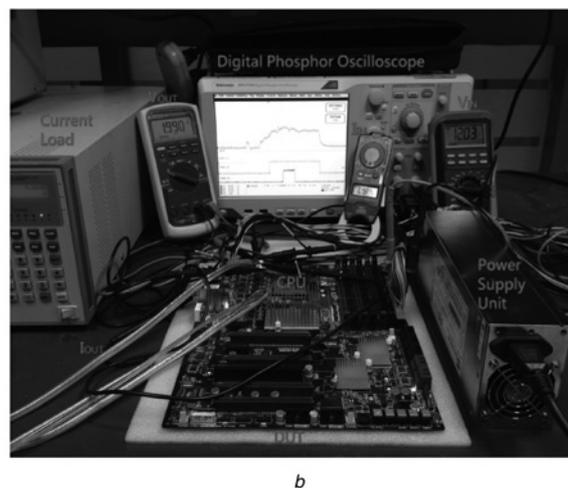
**Fig. 7** Measuring the power conversion efficiency of the PWM regulator
