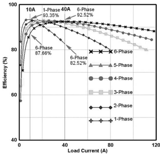
Fig. 1 Multi-phase PWM power conversion efficiency
