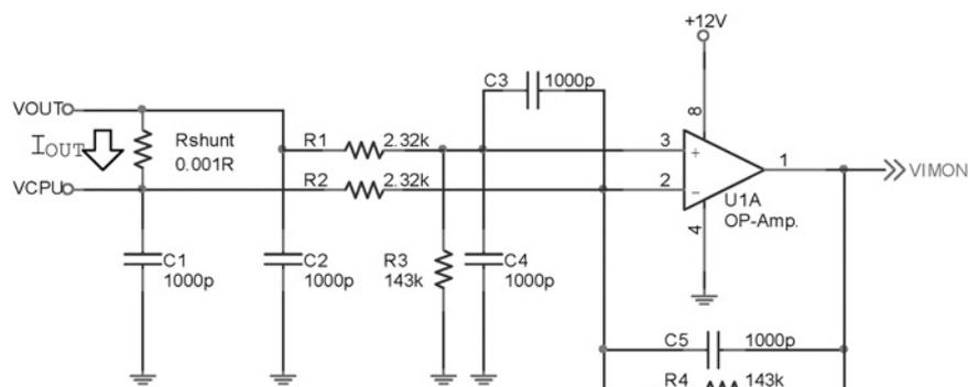
Fig. 3 Output current detection circuit
