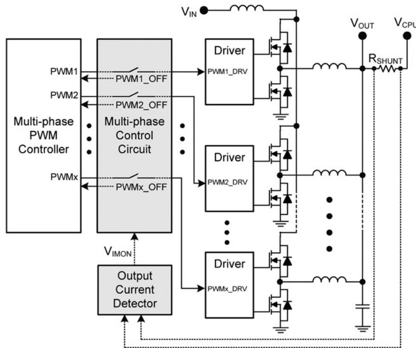
Fig. 2 Block diagram of the multi-phase auto-control method
