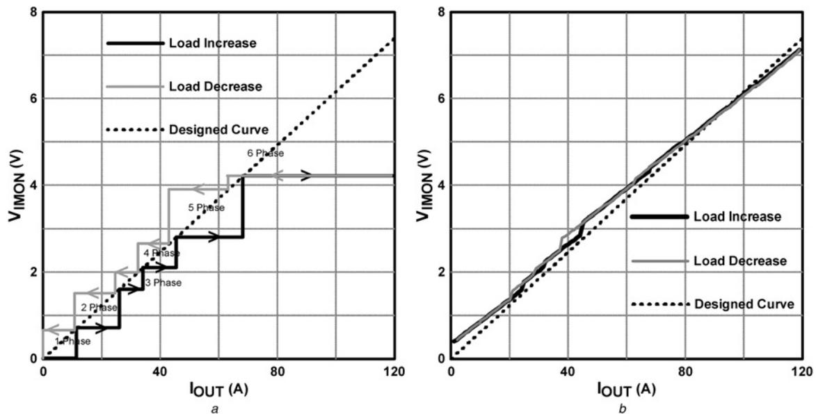
**Fig. 6** Current to voltage conversion curve of the OP-Amp
