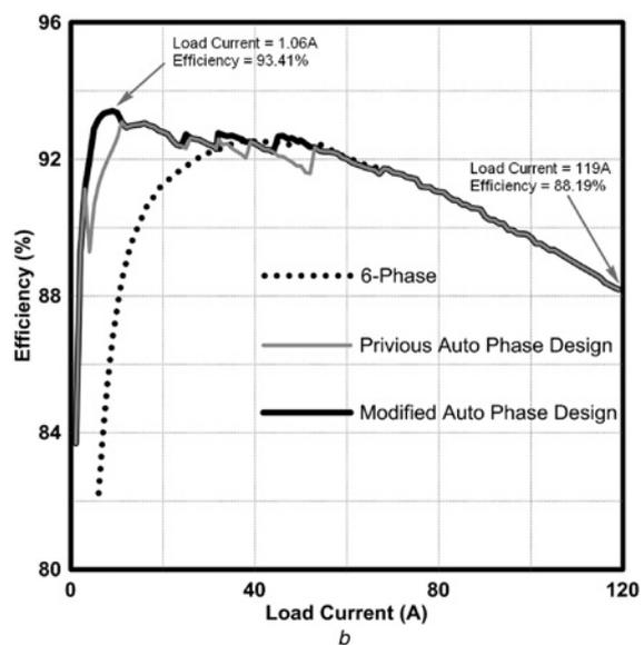
improved from the light load to the heavy load. In this design, the power conversion efficiency can be maintained from 88.19 to 93.41%, when the load current is changed from 1.06 to 119 A. Compared with the traditional fixed multi-phase DC–DC buck regulator design, this flexible multi-phase design increases the power conversion efficiency by  $\sim 2\text{--}23\%$ .
