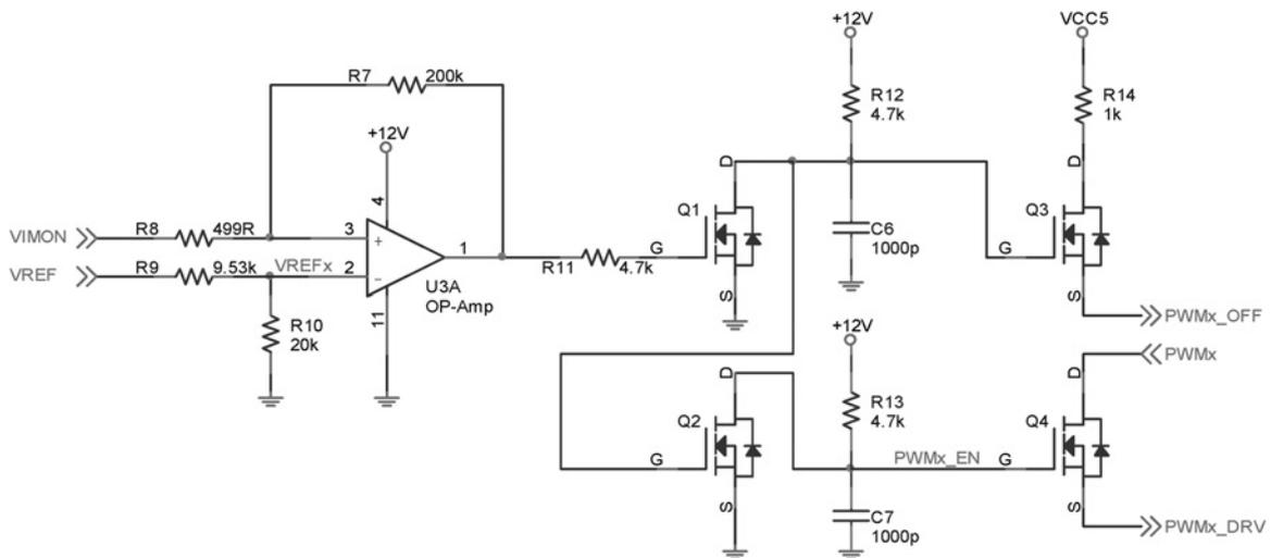
**Fig. 5** Multi-phase control circuit with hysteresis
