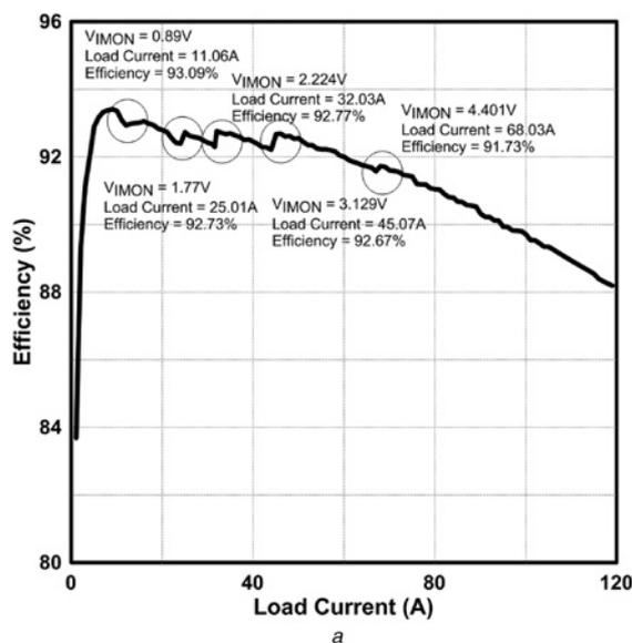
**Fig. 11** Measurement results of the power conversion efficiency
