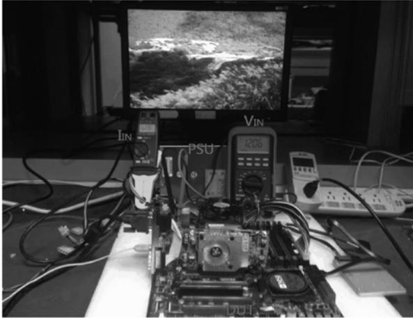
**Fig. 10** Power conversion efficiency measurement
