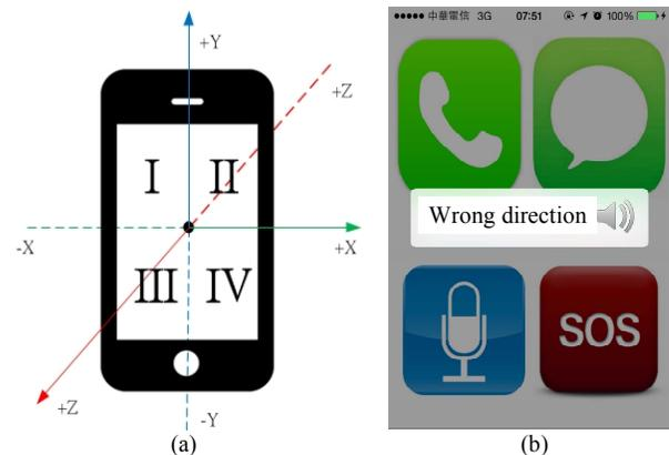
Fig. 3. (a) Smartphone direction (b) Four-quadrant interface with warning message.
