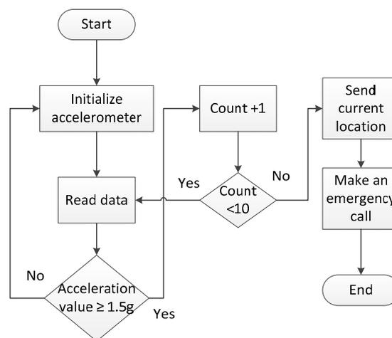
Fig. 6 The flowchart of the emergency function activated by shaking the smartphone.
