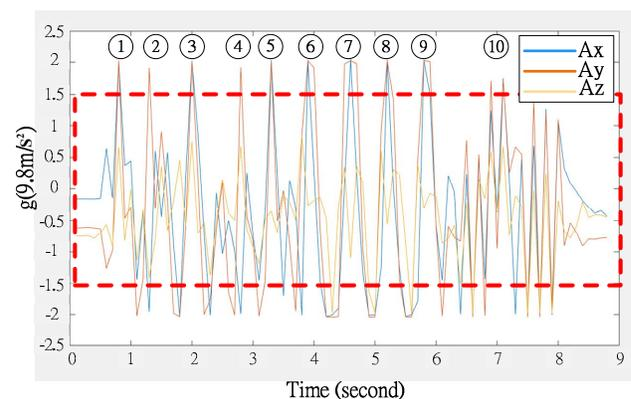
Fig. 5 The acceleration value when a VI user shakes the smartphone more than 10 times.
