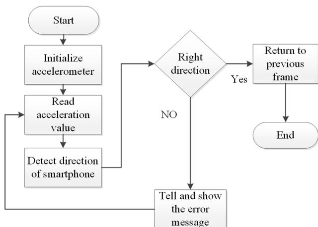
Fig. 4. Smartphone direction detection flowchart.
