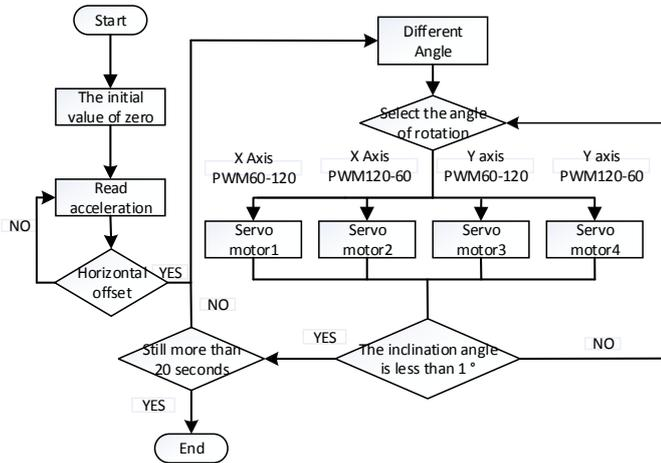
Fig. 3. The ABT software flowchart.
