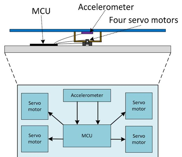
Fig. 2. ABT hardware architecture.
