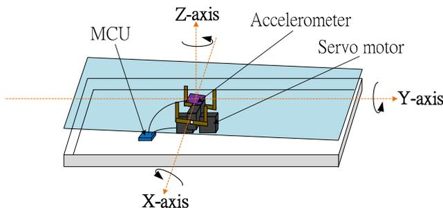
Fig. 1. The definition of roll, pitch, yaw in an automatic balanced tray.
