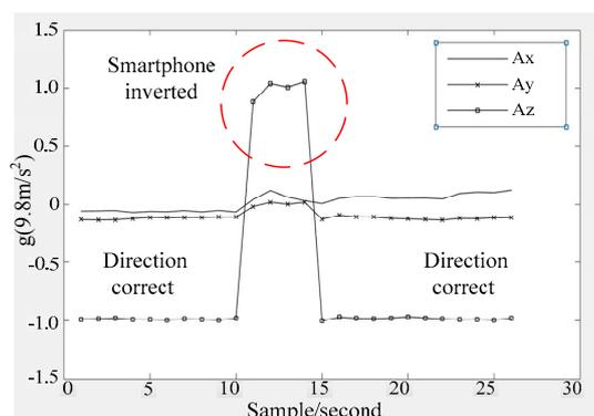
Fig. 4. Acceleration value when the smartphone inverted.
