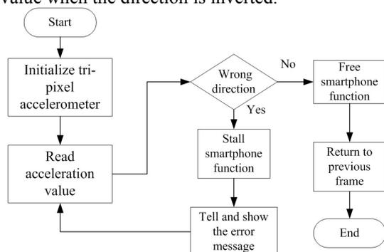
Fig. 3. Direction detection flowchart.
