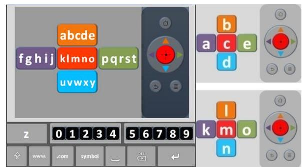
Fig. 1. Left: Full layout of the upper right/lower right on-screen keyboard, after locking on the first key, the user presses either the up button or the enter button on the RC in order that the corresponding direction mini keyboard will appear.
