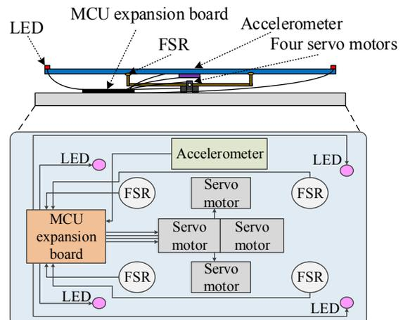
Fig. 2. ADBT hardware architecture.
