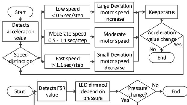
Fig. 4. A flowchart showing the balance sensitivity adjustment process and the reminder function process.
